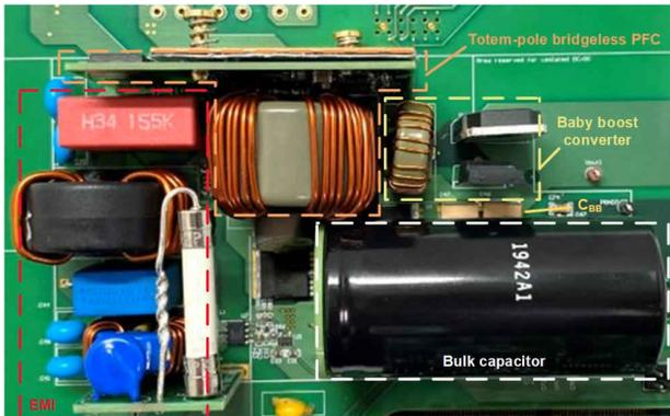
**Figure 3.** 3.6-kW single-phase totem-pole bridgeless PFC reference design with  $>180\text{-W/in}^3$  power density.
