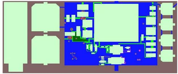
**Figure 2.** Comparing output- and input-side holdup solutions: the input-side holdup solution with one 1,200- $\mu\text{F}$ , 80-V, 16-mm-by-40-mm input capacitor is 4.6 by 1.85 inches – half the size.
