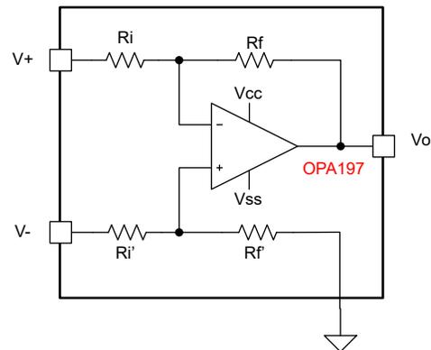
Figure 6. Discrete difference amplifier topology.
