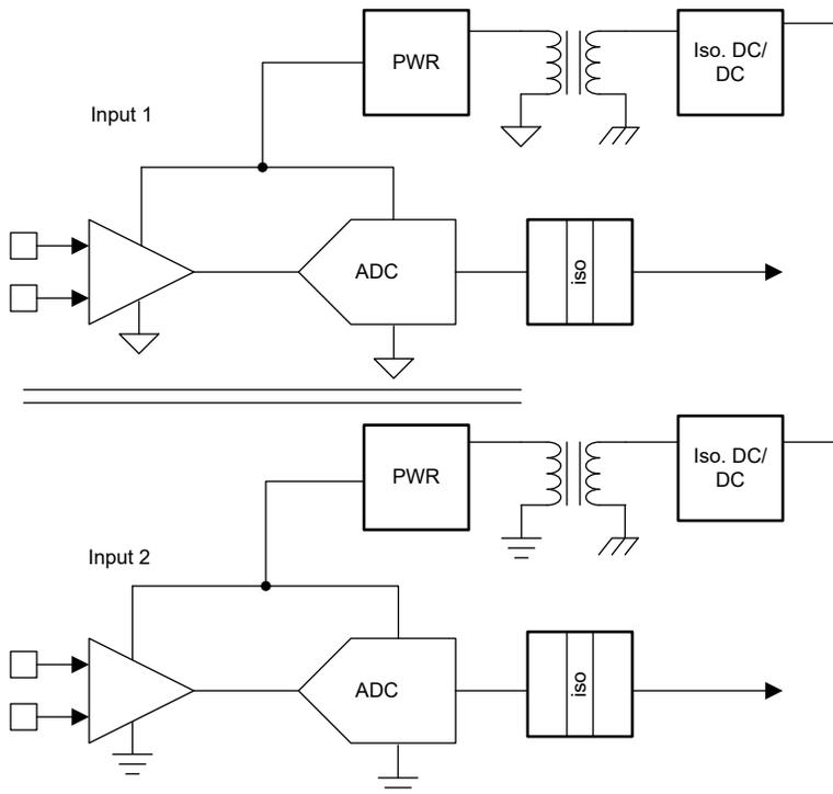
**Figure 2.** Channel-to-channel isolated topology.
