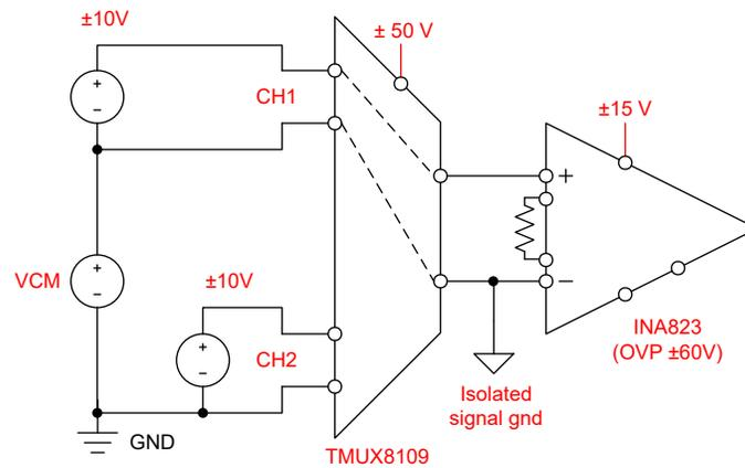
**Figure 3.** High-voltage multiplexer topology block diagram.
