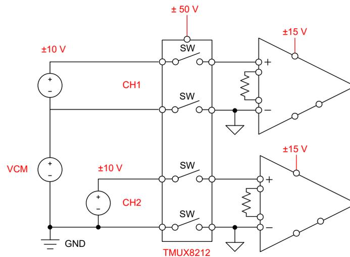
**Figure 4.** High-voltage switch topology block diagram.
