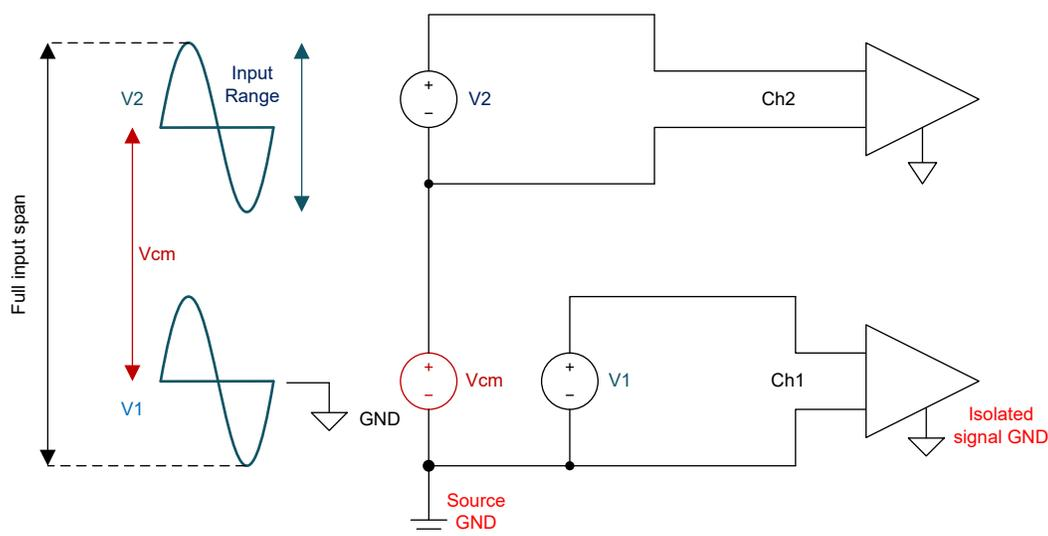
**Figure 1.** Common mode signal absolute input range (full input span): differential input range plus common-mode voltage range.
