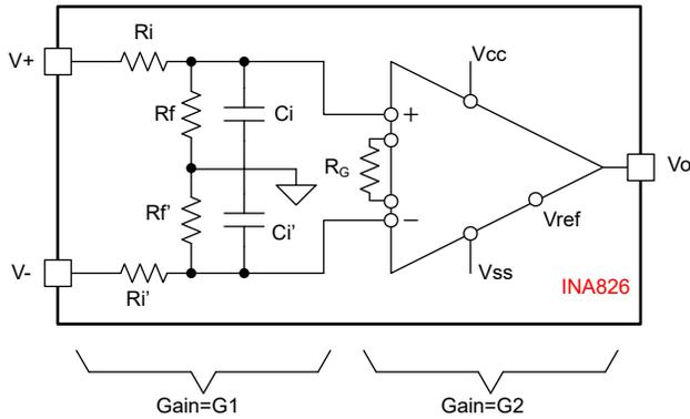
Figure 5. A resistor divider followed by an INA topology.
