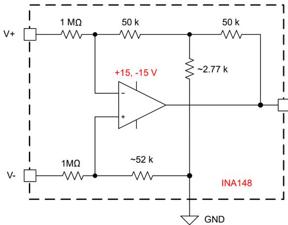
Figure 7. An integrated difference amplifier.
