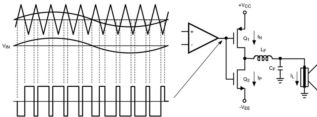
Figure 4. The Class D Audio Amplifier PWM
