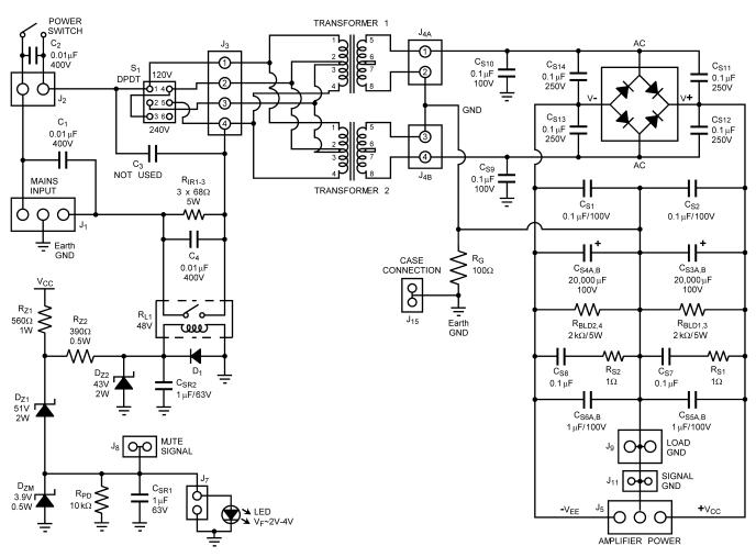
Figure 1. Complete Power Supply Circuit
