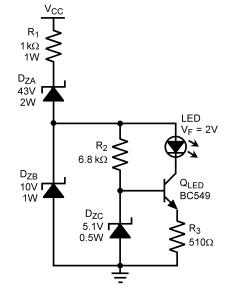
Figure 9. Constant Brightness LED Circuit
