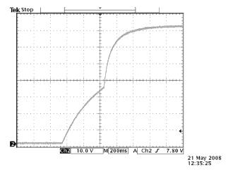
Figure 5. Supply Ramp at Power On
