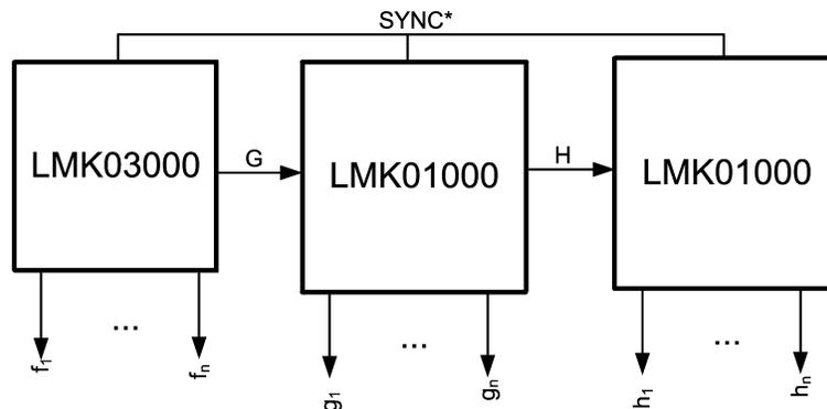
Figure 10. Using the LMK03000 Multiple LMK01000 Devices
