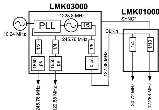
**Figure 8. Using the LMK03000 and LMK01000 Together**
