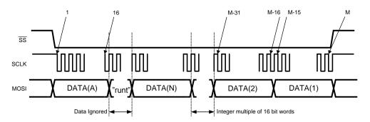
Figure 6. Flexible DAC Bus Cycle
