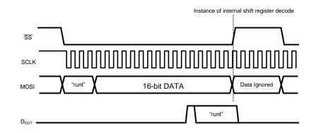
Figure 4. 8-Channel DAC Bus Cycle
