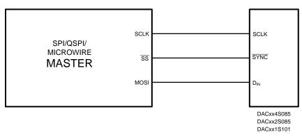
Figure 1. Typical Digital Interface Connectivity
