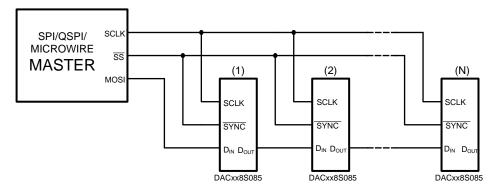
Figure 3. Typical Controller to N 8-Channel DACs Interface: Daisy Chain
