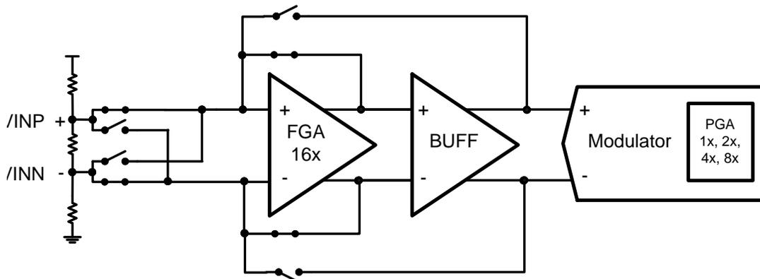
Figure 3. Gain Calibration Technique
