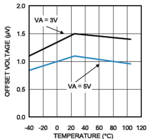
Figure 5. Offset Error at Gain = 1 With Calibration
