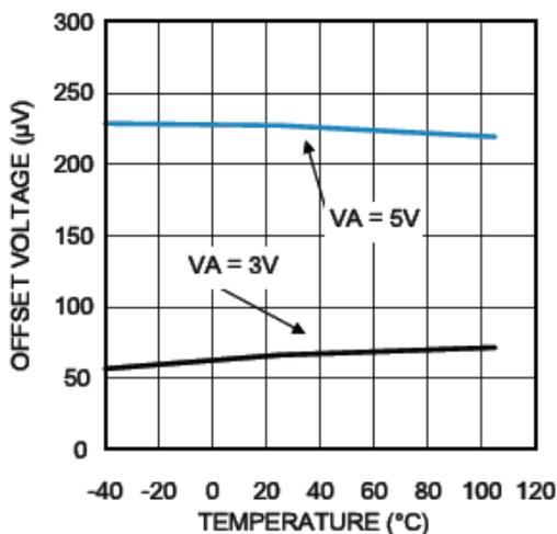
Figure 4. Offset Error at Gain = 1 Without Calibration
