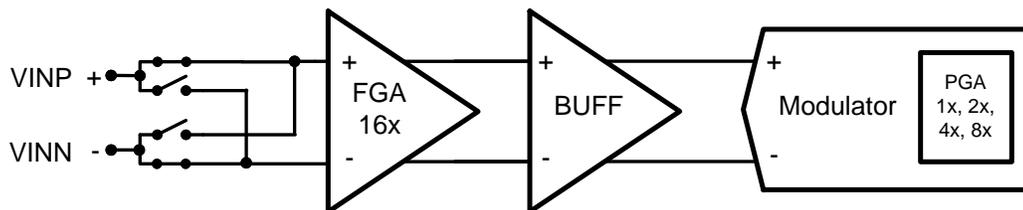
Figure 2. Offset Calibration Technique Diagram
