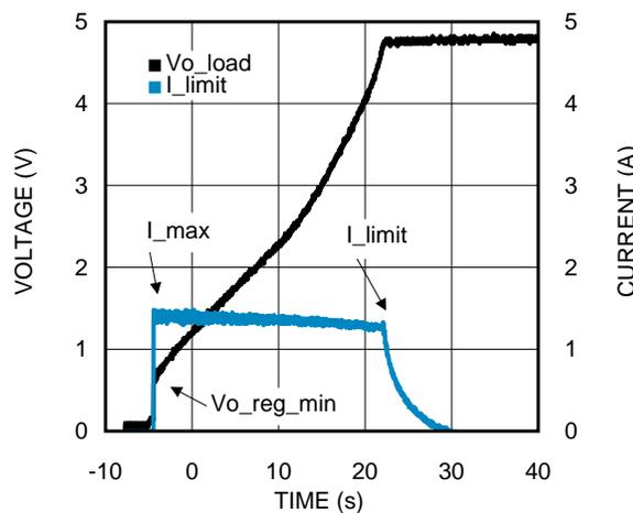
Figure 3. SuperCap Application with LM3102 Regulator Plot
