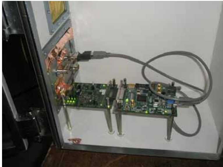
Photograph 7.1.4 Setup for radiated disturbance measurements, EUT close view
