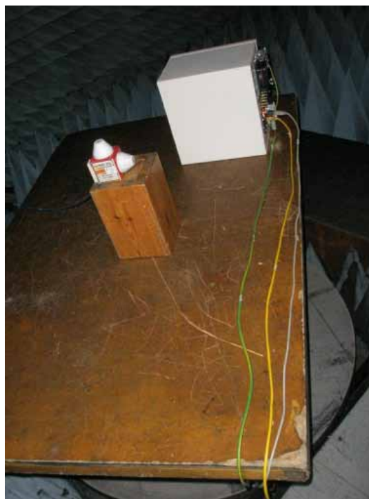
Photograph 8.1.2 Setup for radiated immunity to RF electromagnetic field test, EUT close view, EUT radiation through cable
