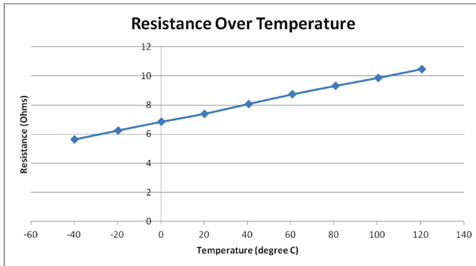
Figure 1. Resistance of a Typical PCB Coil as a Function of Temperature
