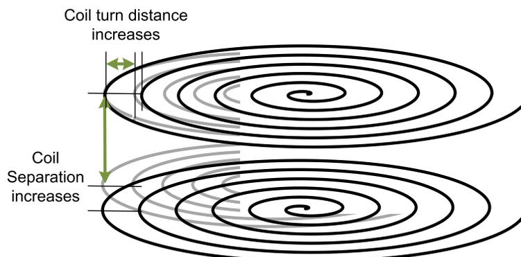
Figure 2. Multi-Layer Coil Geometry Shift Due to Temperature
