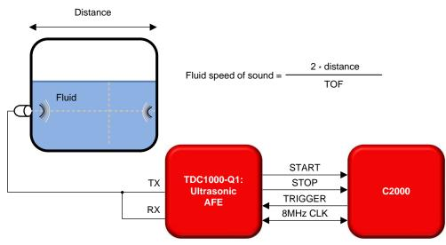
Figure 1. Fluid Identification Block Diagram
