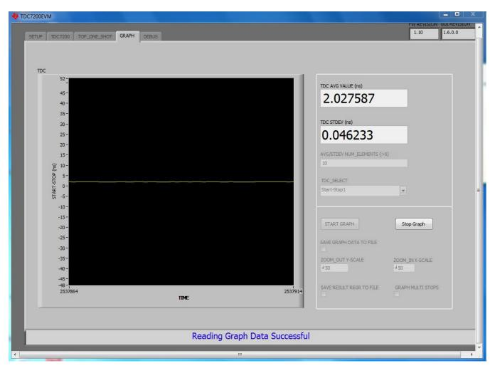
Figure 12. TDC7200 Interleaved Short Time Measurement Results
