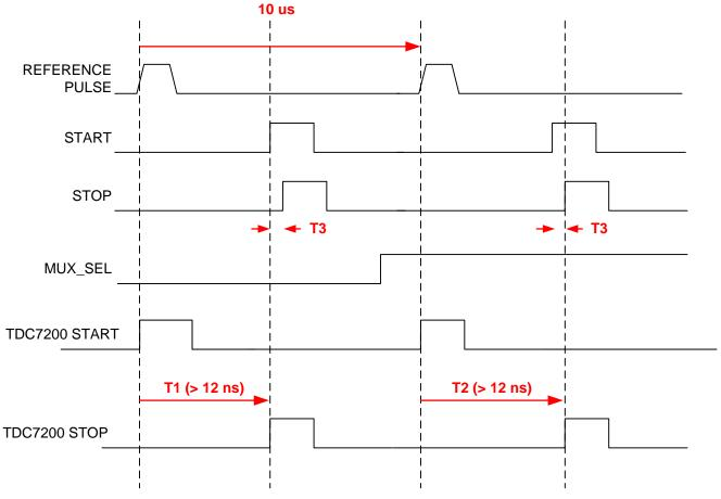
Figure 6. Interleaved Short Time Measurements Timing Diagram
