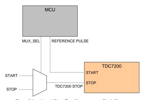
Figure 5. Interleaved Short Time Measurements Block Diagram
