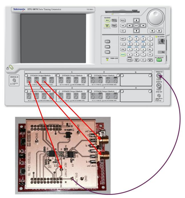
Figure 10. DTG5078 Based Test Setup
