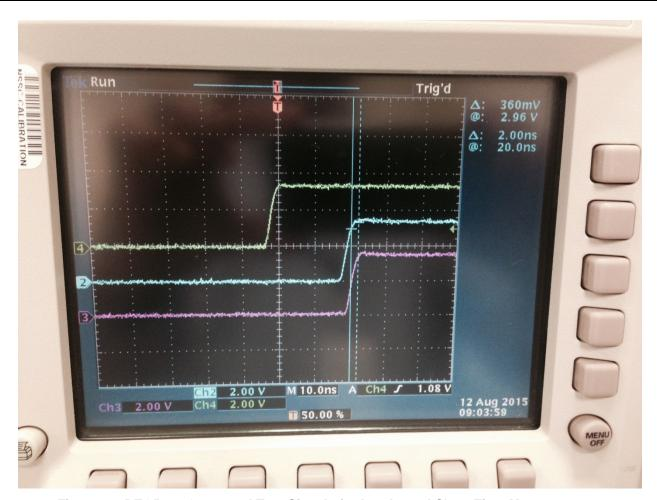
Figure 11. DTG5078 Generated Test Signals for Interleaved Short Time Measurements
