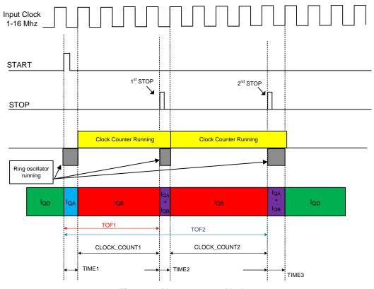
Figure 4. Measurement Mode 2
