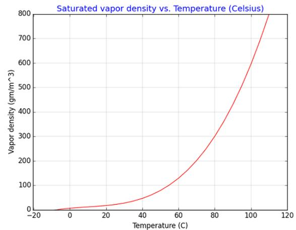
**Figure 1. Saturated Vapor Density vs Temperature Graph** <sup>(1)</sup>
