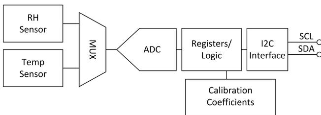
**Figure 3. Relative Humidity and Temperature Sensor Block Diagram**
