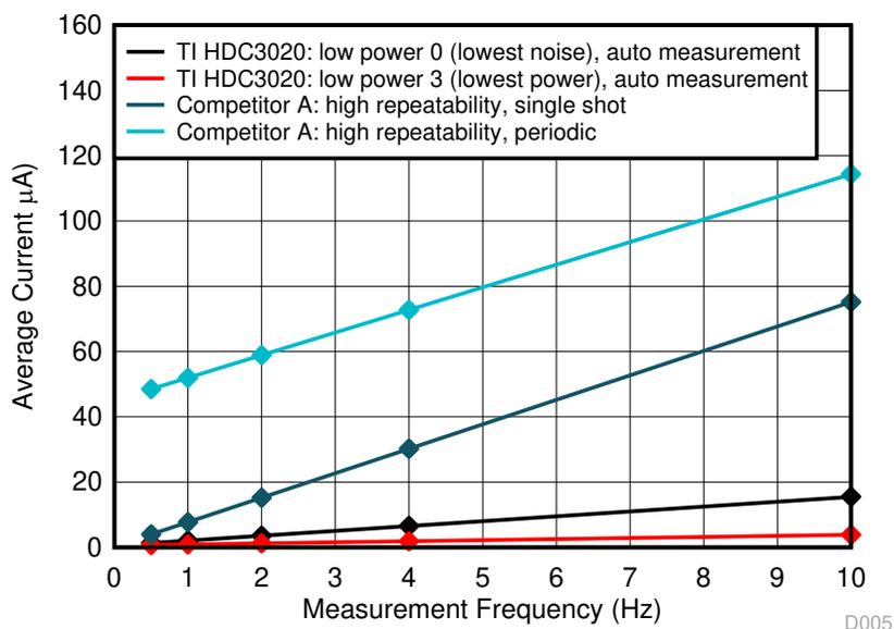
**Figure 3. Competitive Comparison Average Current vs Measurement Frequency**
