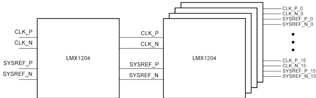
**Figure 1-1. Simple Block Diagram of Cascaded LMX1204 Design**
