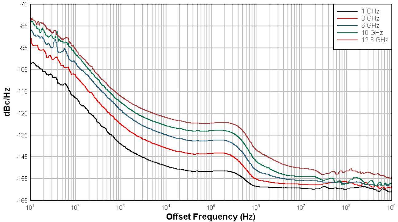
**Figure 2-2. Cascaded LMX1204 Phase Noise Measurements**
