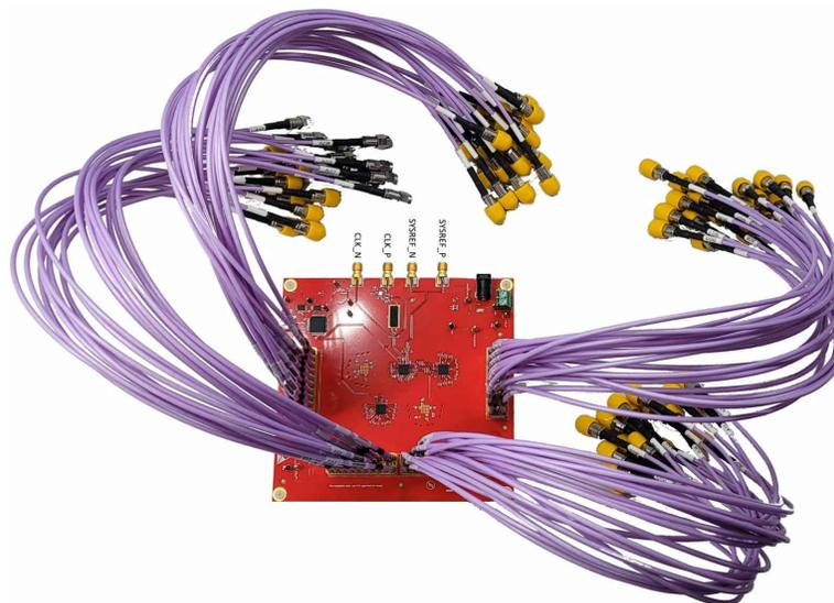
**Figure 1-2. LMX1204 Clock Distribution Board**
