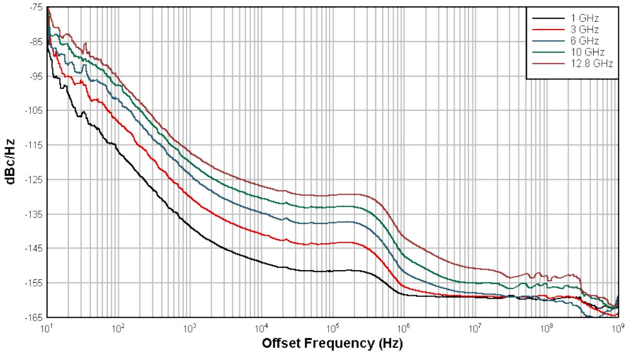
**Figure 2-1. LMX1204EVM Phase Noise Measurements**
