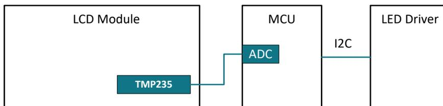
**Figure 3. Using Analog Temperature ICs for Display Temperature Sensing**
