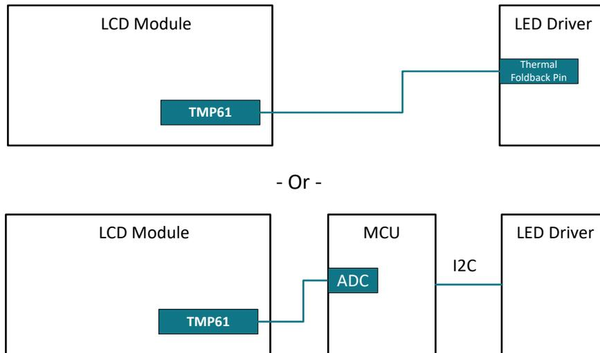
**Figure 2. Using a Thermistor for Display Temperature Sensing**
