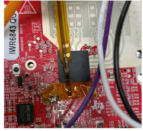
Figure 4-8. TMP114 and TMP117 Temperature Sensor Testing Setup
