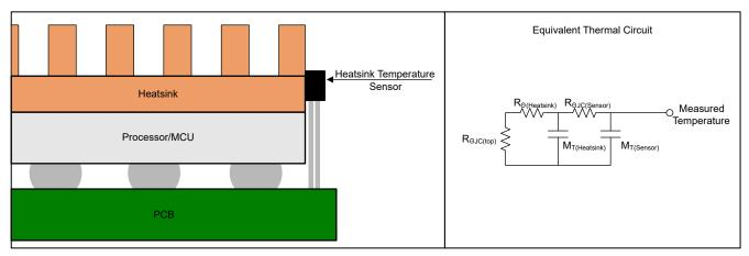
Figure 2-1. Equivalent Thermal Circuit for Heat Sink Temperature Sensing
