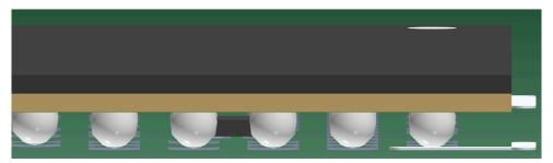
Figure 4-3. Board Rendering of TMP114 Temperature Sensor Underneath IWR6843 Sensor
