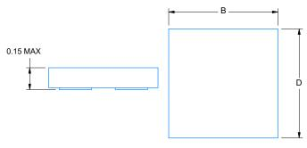
Figure 4-2. TMP144 and TMP144 YMT Package Drawing
