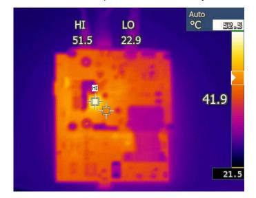
Figure 4-1. Thermal Capture of AWR2243BOOST Under Moderate Load
