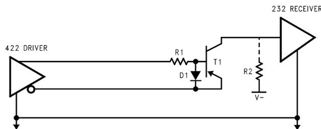
Figure 3. RS-422 to RS-232—with Active Device
