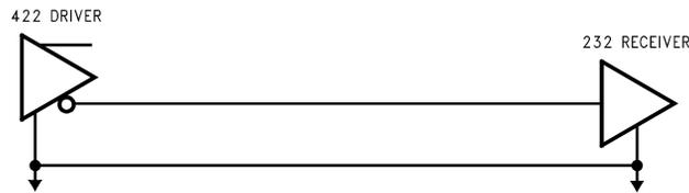
**Figure 4. RS-422 to RS-232—Direct Connection**
