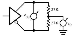
Figure 2. Termination Load Configuration
