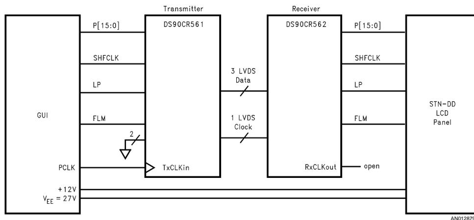
FIGURE 1. STN-DD Panel Application Using FPD-Link Chipset
