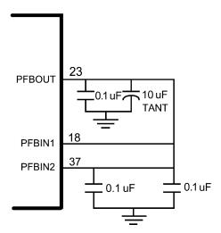
Figure 1. Special Connection in DP83848C/I/YB
