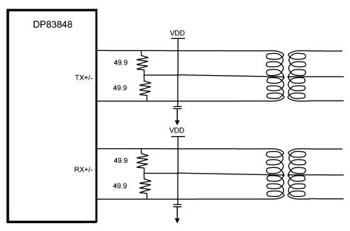
Figure 2. DP83848C/I/YB PMD Connections (Termination and Biasing)
