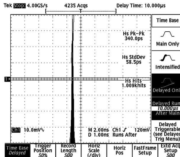
Figure 2. 10 µs Delay Jitter Histogram With FCO Source
