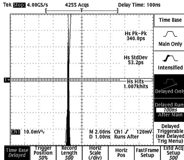
Figure 3. Cycle-to-Cycle Jitter Histogram With PGM Source
