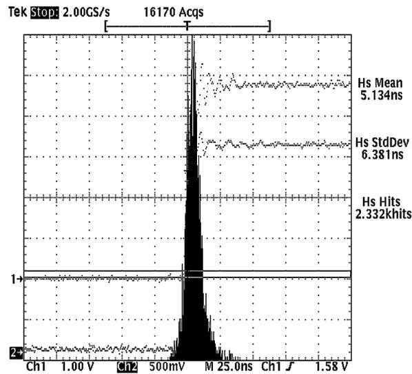
Figure 6. Clock Output Phase Error With PGM Source
