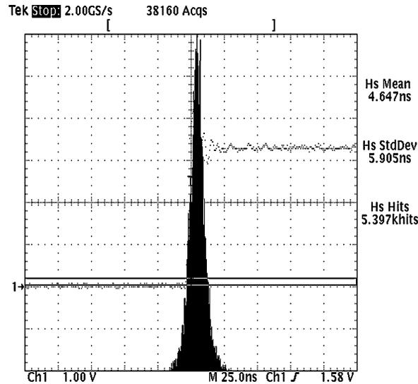
Figure 5. Clock Output Phase Error With FCO Source
