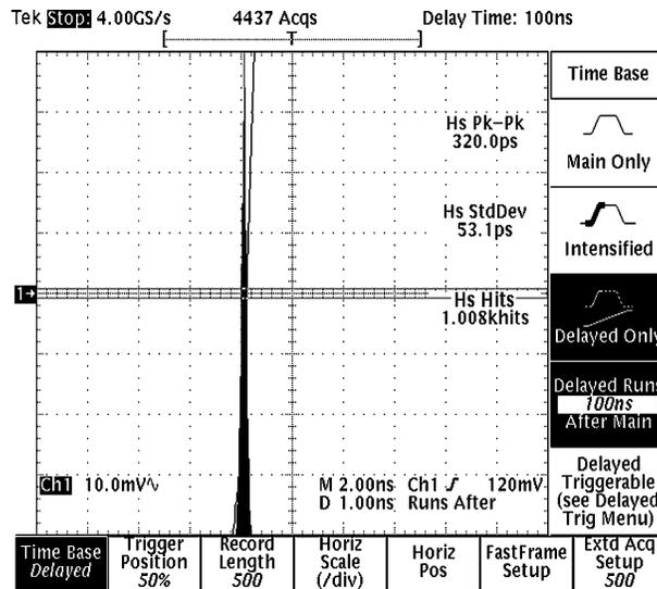
Figure 1. Cycle-to-Cycle Jitter Histogram With FCO Source
