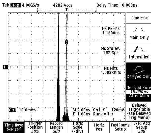
Figure 4. 10 µs Delay Jitter Histogram With PGM Source
