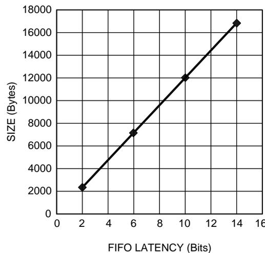
**Figure 1. FIFO Latency vs. Maximum Packet Size**
