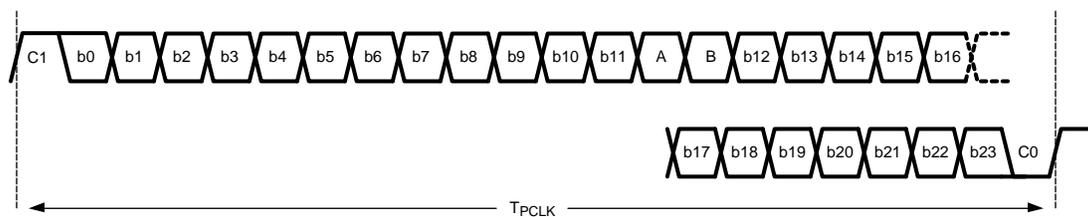
**Figure 2. 24-bit Serial Payload Example**
