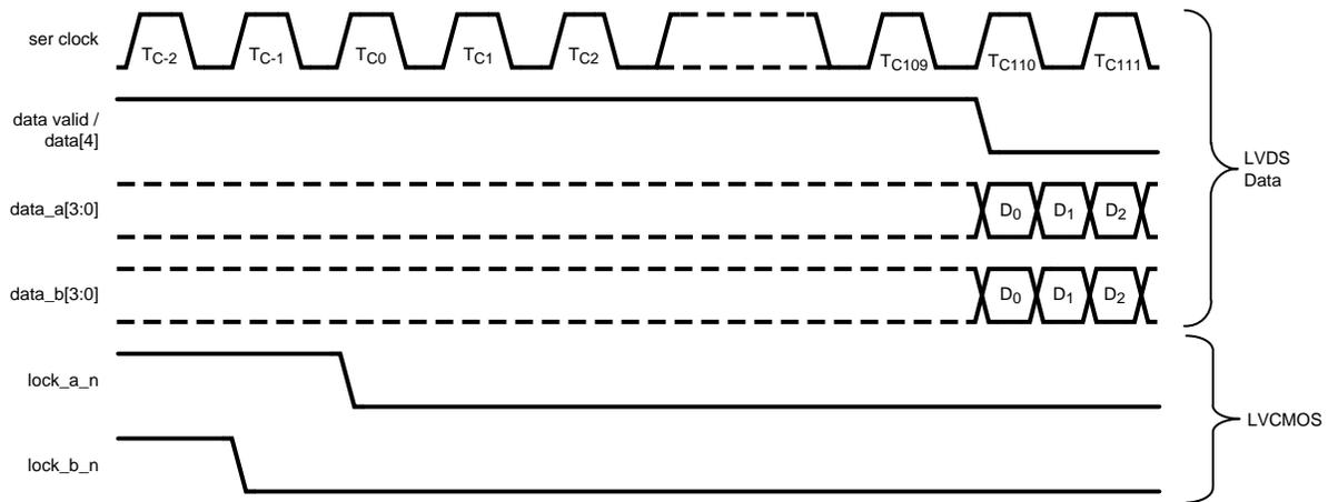
Figure 4. FPGA to Serializer Interface Two Links
