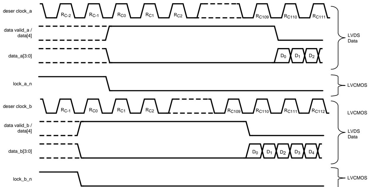
Figure 5. FPGA to Deserializer Interfaces Two Links
