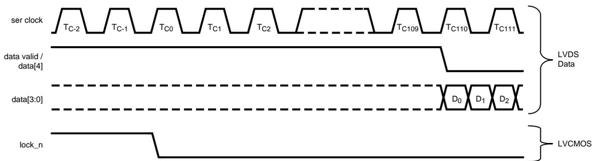
Figure 2. FPGA to Serializer Interface Single Link
