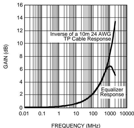
Figure 2. Response of a Peaking Equalizer with the Center Frequency at 1 GHz Closely Matches the Inverse of a 10m 24 AWG Twisted Pair Cable Response
