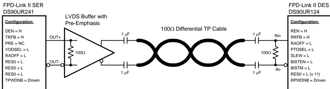
**Figure 6. Connection Diagram with a Buffer with Integrated Pre-emphasis Circuit**
