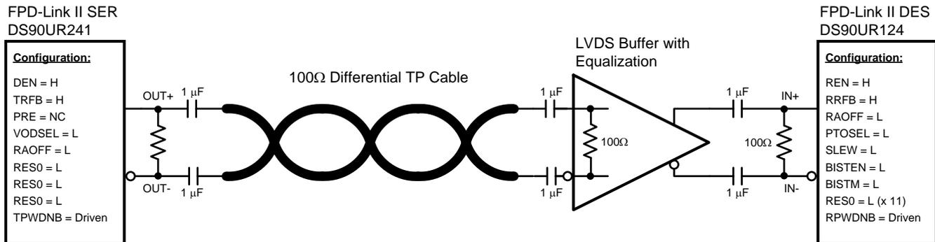
Figure 7. Connection Diagram with a Buffer with Integrated Equalizer Circuit
