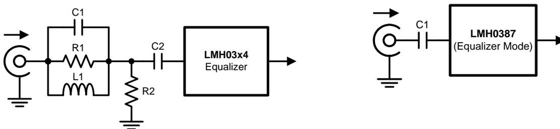
**Figure 3. Input Circuit Required for Dedicated Equalizer (left) and LMH0387 (right)**
