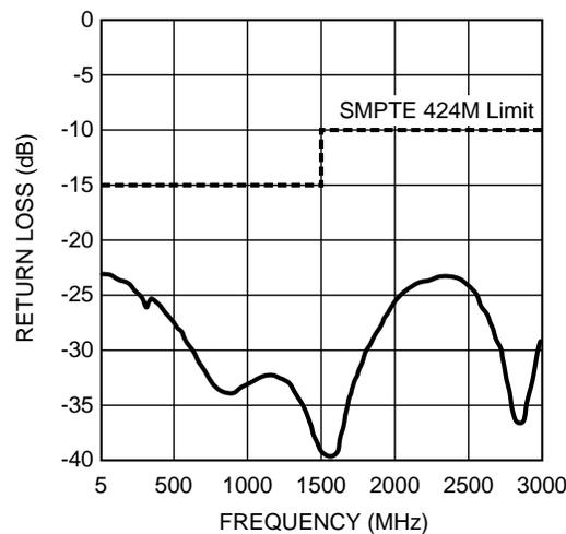
**Figure 2. LMH0387 Input Return Loss**
