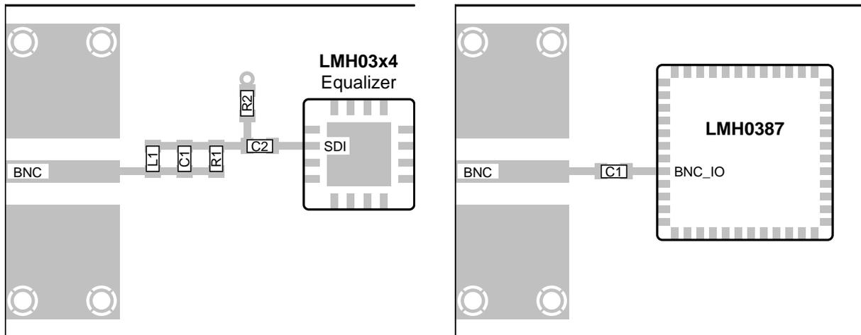
**Figure 4. Input Circuit PCB Layout for Dedicated Equalizer (left) and LMH0387 (right)**
