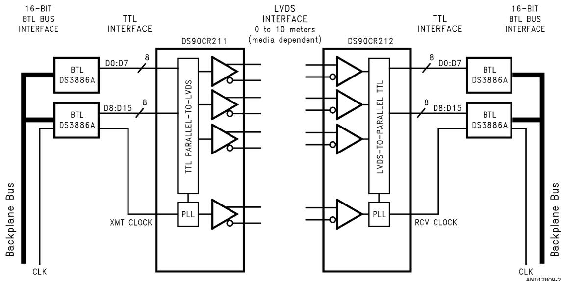
FIGURE 2. CHANNEL LINK 16-Bit Bus Extension
