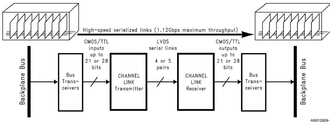
FIGURE 1. CHANNEL LINK Subsystem Communications Solution
