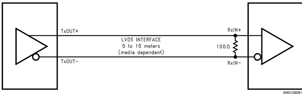
FIGURE 9. LVDS Serialized Link Termination
