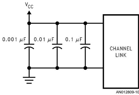
**FIGURE 10. CHANNEL LINK Decoupling Configuration**
