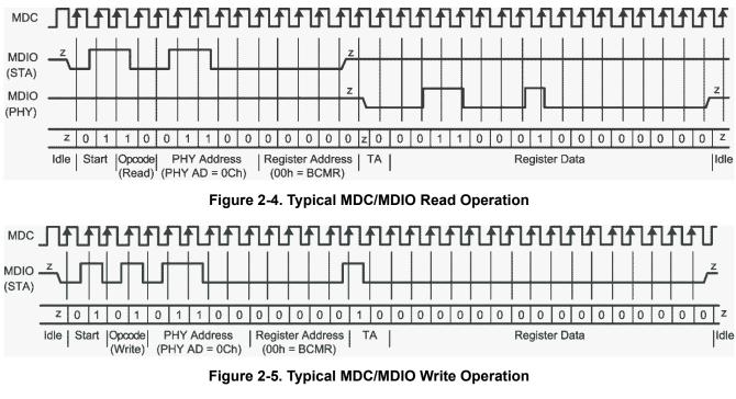
**Note** Recommend using Logic Analyzer to debug MDIO communication.
