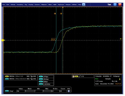
Figure 2-13. 10Mbps Data and Clock Delay in Align Mode
