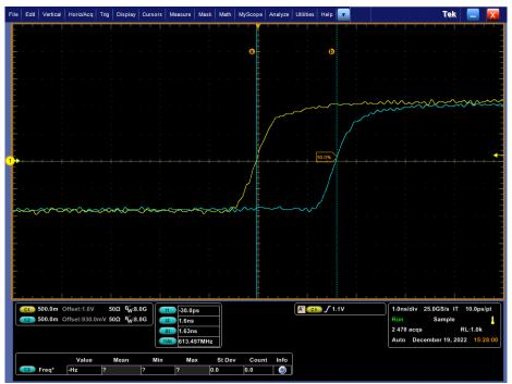
Figure 2-14. 10 Mbps Data and RX\_CLK in Shift Mode (4ns Programmed Delay)
