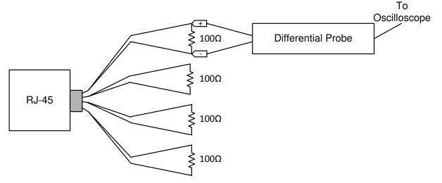
Figure 2-7. Connection Diagram for 100M Terminated Cable
