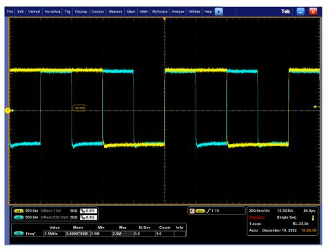
Figure 2-11. 10 Mbps Data Aligned with RX\_CLK
