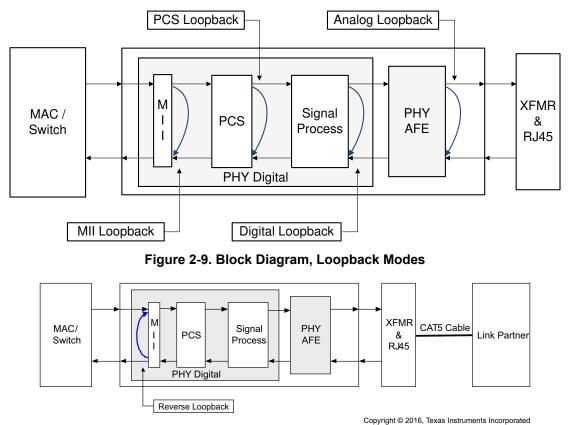
Figure 2-10. Block Diagram, Reverse Loopback Mode
