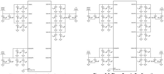
Figure 2-1. Two Supply Configuration
