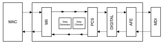
If generating and checking packets with the MAC is not possible, use PRBS packet generation and checking functionalities to verify the data path. Perform reverse loopback with PRBS and a working link partner as follows:
