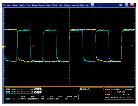
Figure 2-12. 100 Mbps Data Aligned with RX\_CLK
