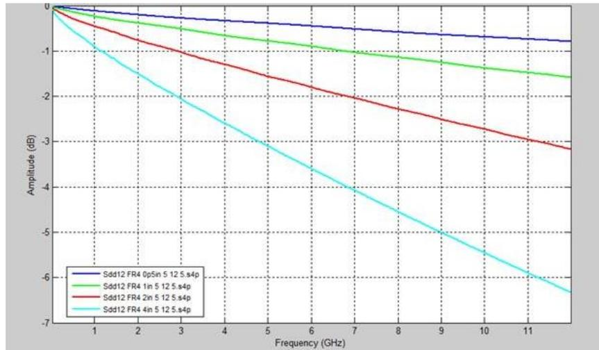
Figure 1. FR4 SDD21 Insertion Loss vs Frequency for Various Trace Lengths
