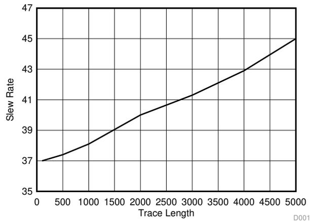
Figure 2. FR4 Slew Rate (ps) vs Trace Lengths (mils)
