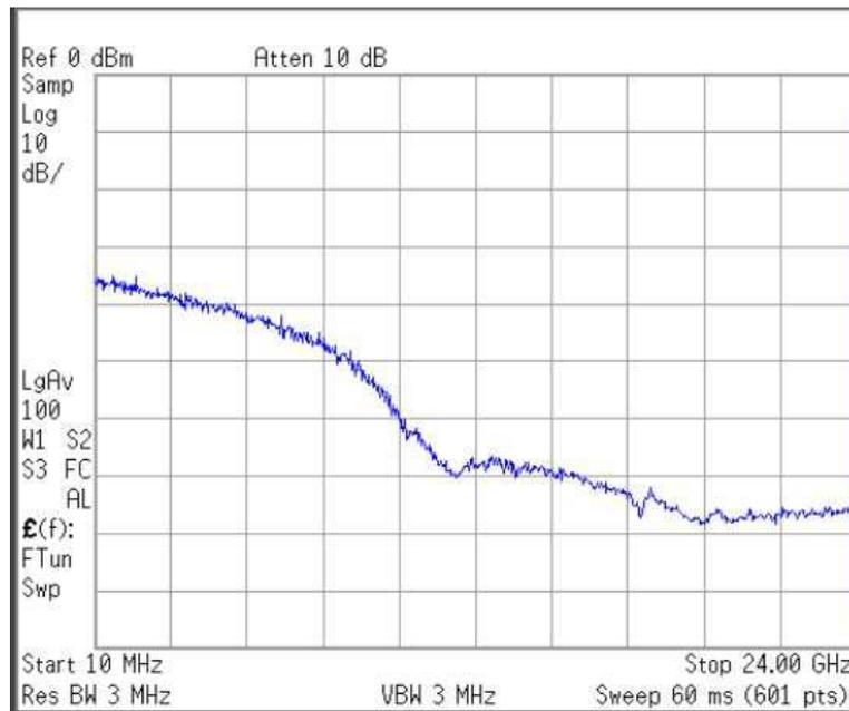
Figure 7. 12G Video Pattern Spectrum (2.4 GHz/div.)
