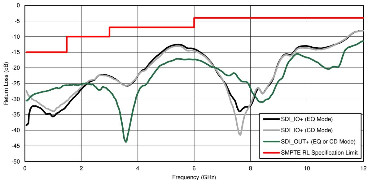
Figure 3. LMH1297 Return Loss without External Components
