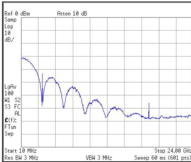
Figure 6. 3G Video Pattern Spectrum (2.4 GHz/div.)
