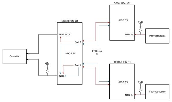
Figure 10-2. Interrupt Propagation in Splitter Mode Block Diagram
