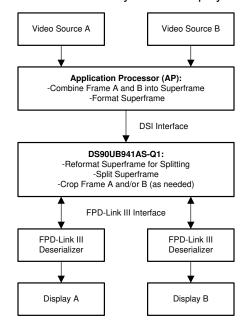
Figure 1-1. Superframe Creation and Splitting System Block Diagram
