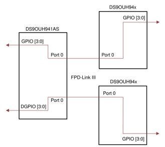
Figure 11-1. Splitter Mode GPIO Block Diagram
