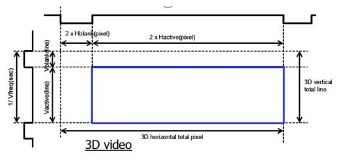
Figure 2-3. HDMI 1.4b Alternate Pixel 3D Format
