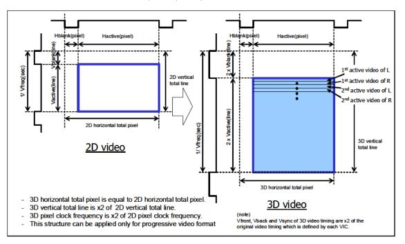
Figure 2-2. HDMI 1.4b Alternate Line 3D Format
