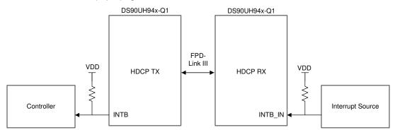
Figure 10-1. Receiver Interrupt Propagation Block Diagram
