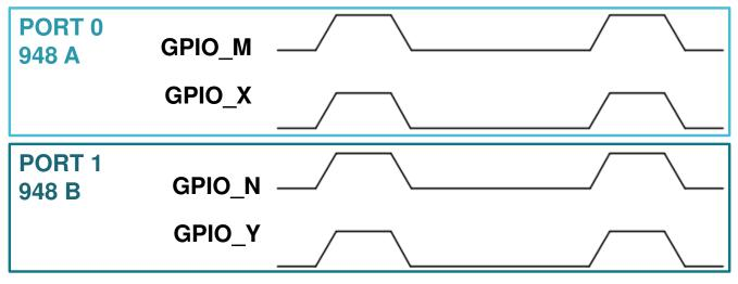
Figure 10-6. Example GPIO Logic with Standard GPIO Pass-Throughs
