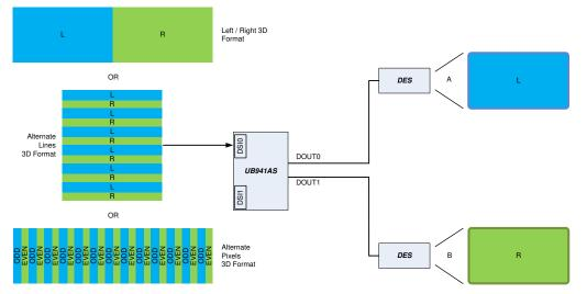
Figure 4-1. Symmetric Splitting
