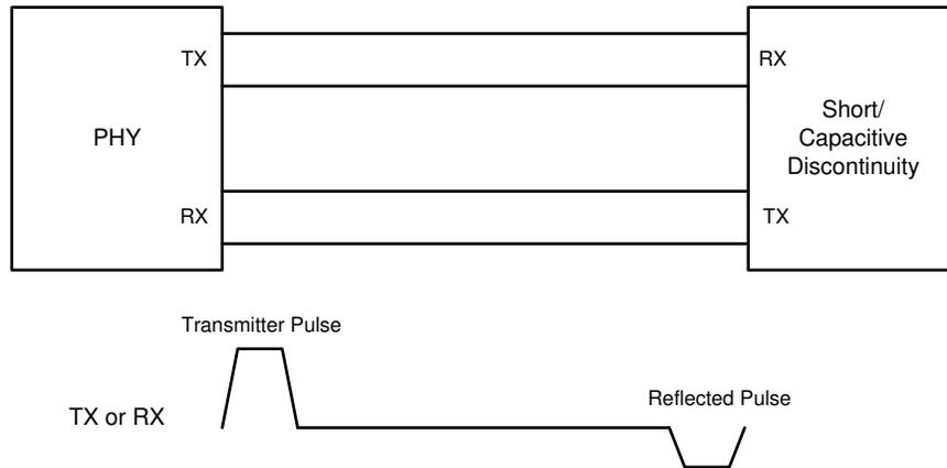
**Figure 2. Short Circuit Cable**
