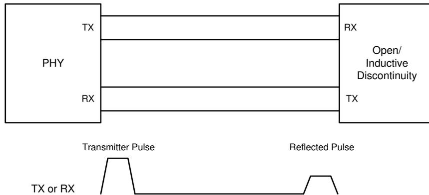
**Figure 1. Open Circuit Cable**
