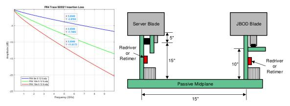
Figure 2-2. IL Increases with Frequency While PCB Distance Remains the Same
