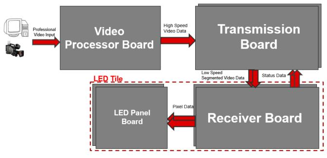
Figure 2-1. LED Wall Functional Block Diagram
