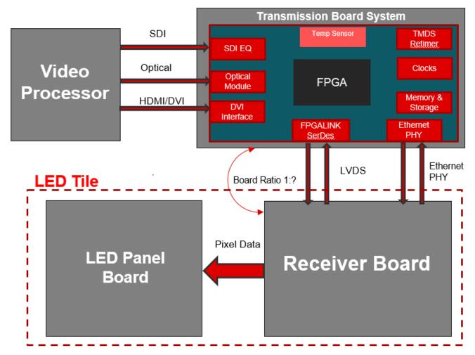
Figure 2-3. Transmission Board
