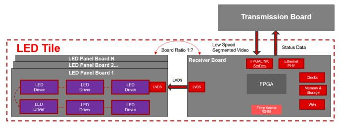
Figure 2-5. Receiver Board
