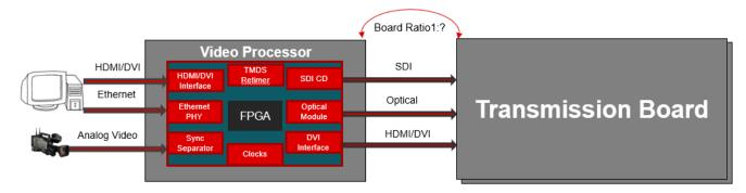
Figure 2-2. Processor Board
