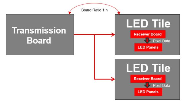
Figure 2-4. Daisy Chained Transmission Board
