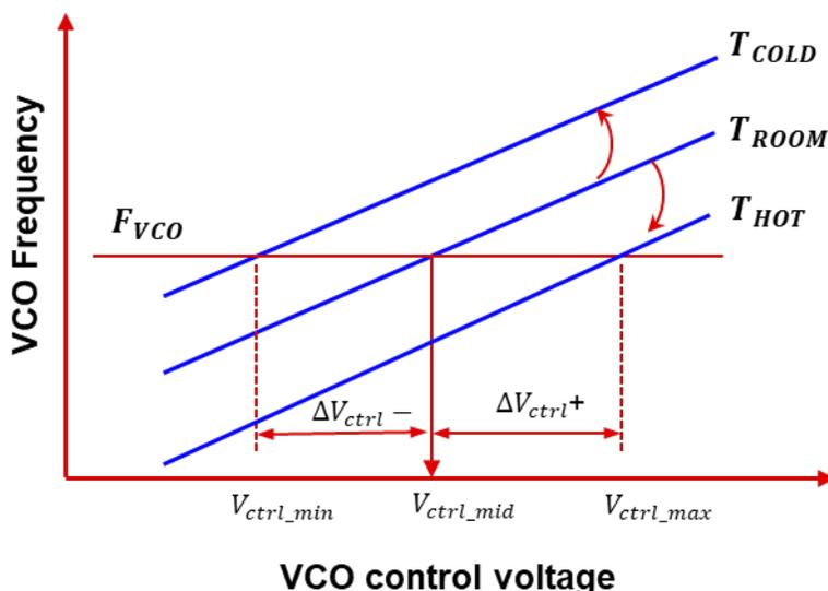
**Figure 3-1. Impact of Temperature on VCO Frequency**
