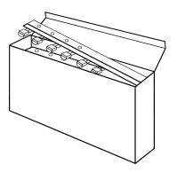
Figure 7. LFT3 Radial Ammo Pack Ammo Pack equivalent to option LFT1. Flat side of transistor on adhesive side of tape.
