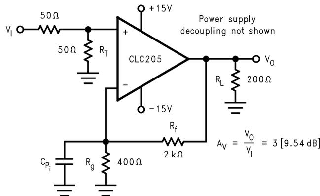
Figure 4. Simulation Circuit for Inverting Input Capacitive Test
