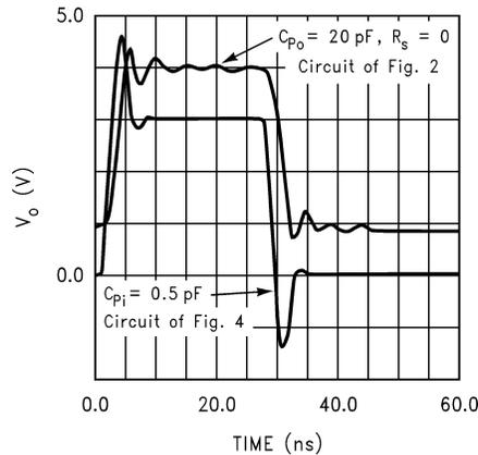
Figure 7. Contrasting Pulse Responses for  $C_{po}$  and  $C_{pi}$
