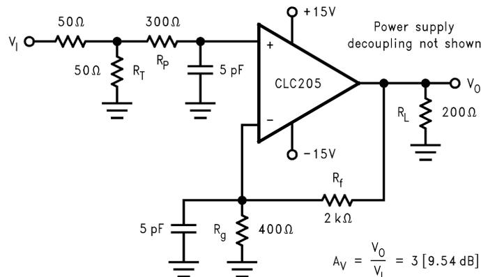
Figure 8. Simulation Circuit of  $C_{pi}$  Peaking Cancellation
