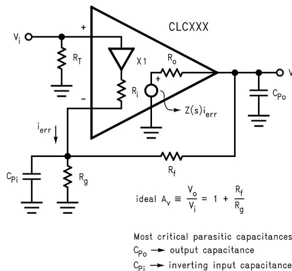
**Figure 1. Non-inverting Gain with Internal Current Feedback Topology**
