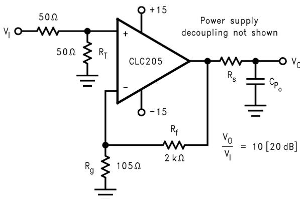
Figure 2. Simulation Circuit for Capacitive Loading Test
