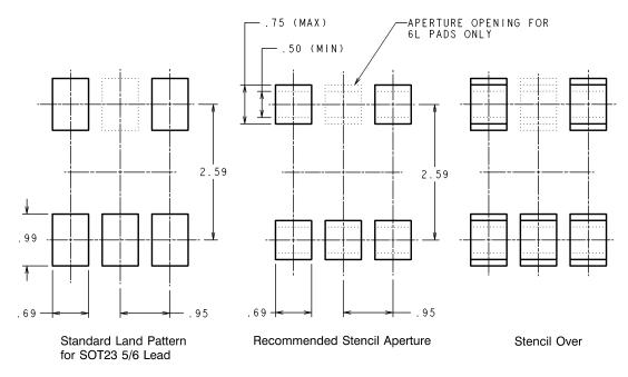
Figure 31. Recommended Stencil Apertures for SOT23 5/6 Lead Footprint Compatible LLP
