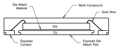
Figure 1. Pullback LLP Configuration
