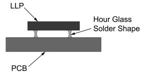
Figure 25. Pullback LLP Hour Glass Solder Joint
