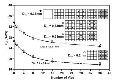
Figure 11.  $\theta_{JA}$  vs. Number, Distribution and Diameter of Thermal Vias and Die Sizes for 36L LLP with 9 × 9 mm Body and 7 × 7 mm Pad
