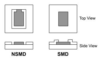
Figure 4. NSMD and SMD Pad Geometry
