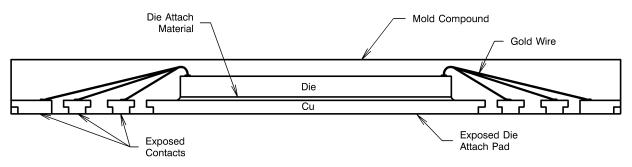
Figure 2. Pullback LLP Configuration with Power and Ground Rings
