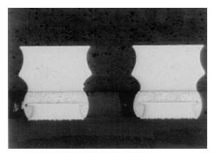
Figure 28. X-section Across Solder Joints
