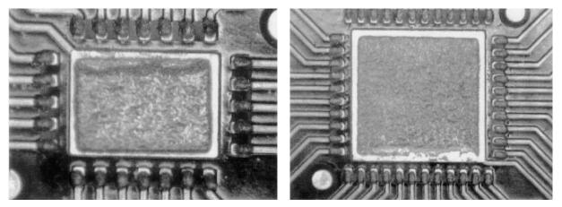
Figure 27. Solder Paste Printing of LLP 24 and LLP 44 Using 127 µm (5 mil) Thick Stencil
