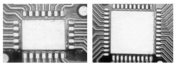
Figure 26. Pads After Removing Components and Cleaning
