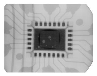
Figure 24. Typical X-ray After Process
