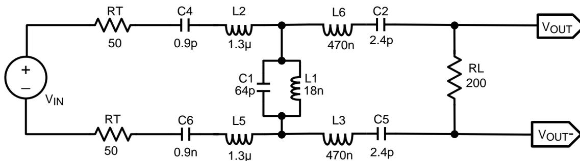
Figure 4. Butterworth Filter with 100Ω Input and 200Ω Output Impedances
