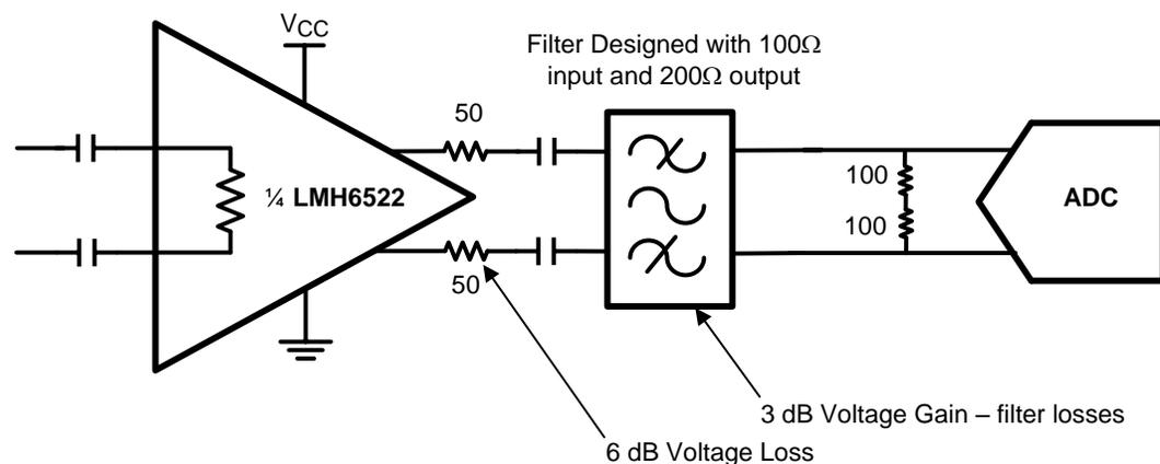
**Figure 2. Using Impedance Transform to Realize Voltage Gain**
