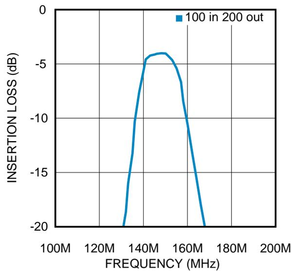
Figure 3. Frequency Response for Impedance Transform Filter
