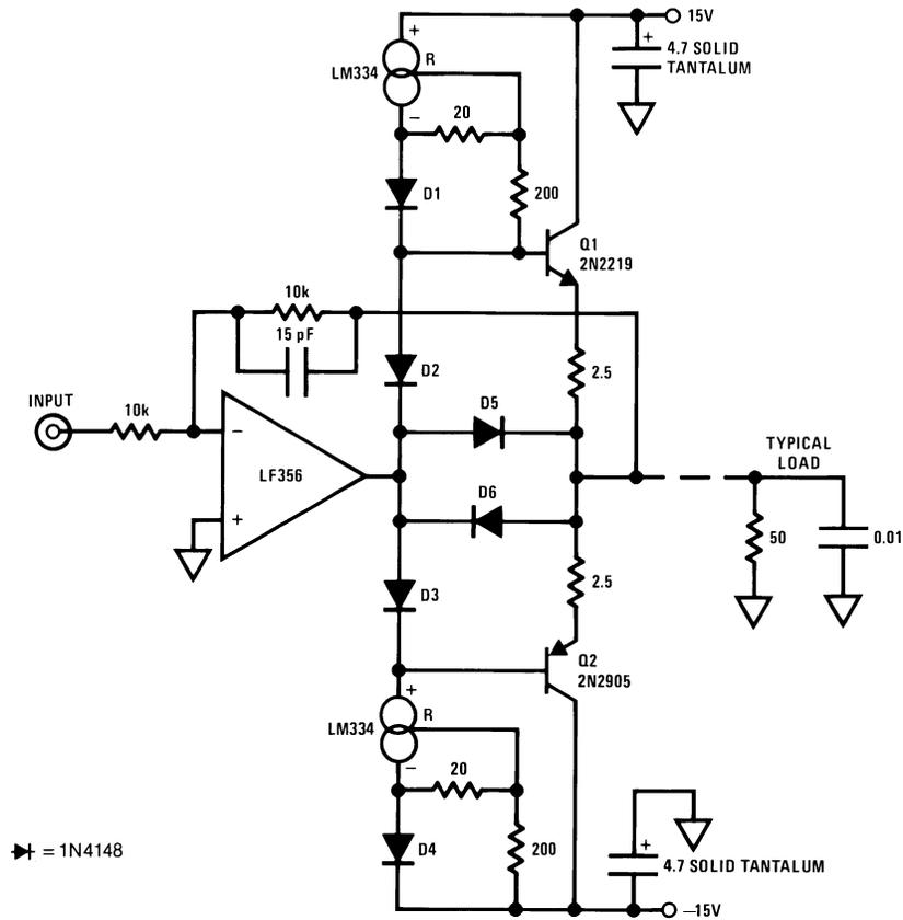
Use TO-5 heat sinks on transistors
