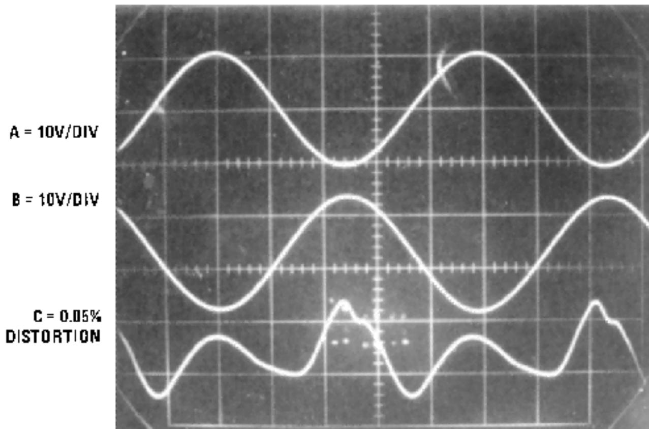
**Figure 2. 100 kHz 20 Vp-p Sine Wave**
