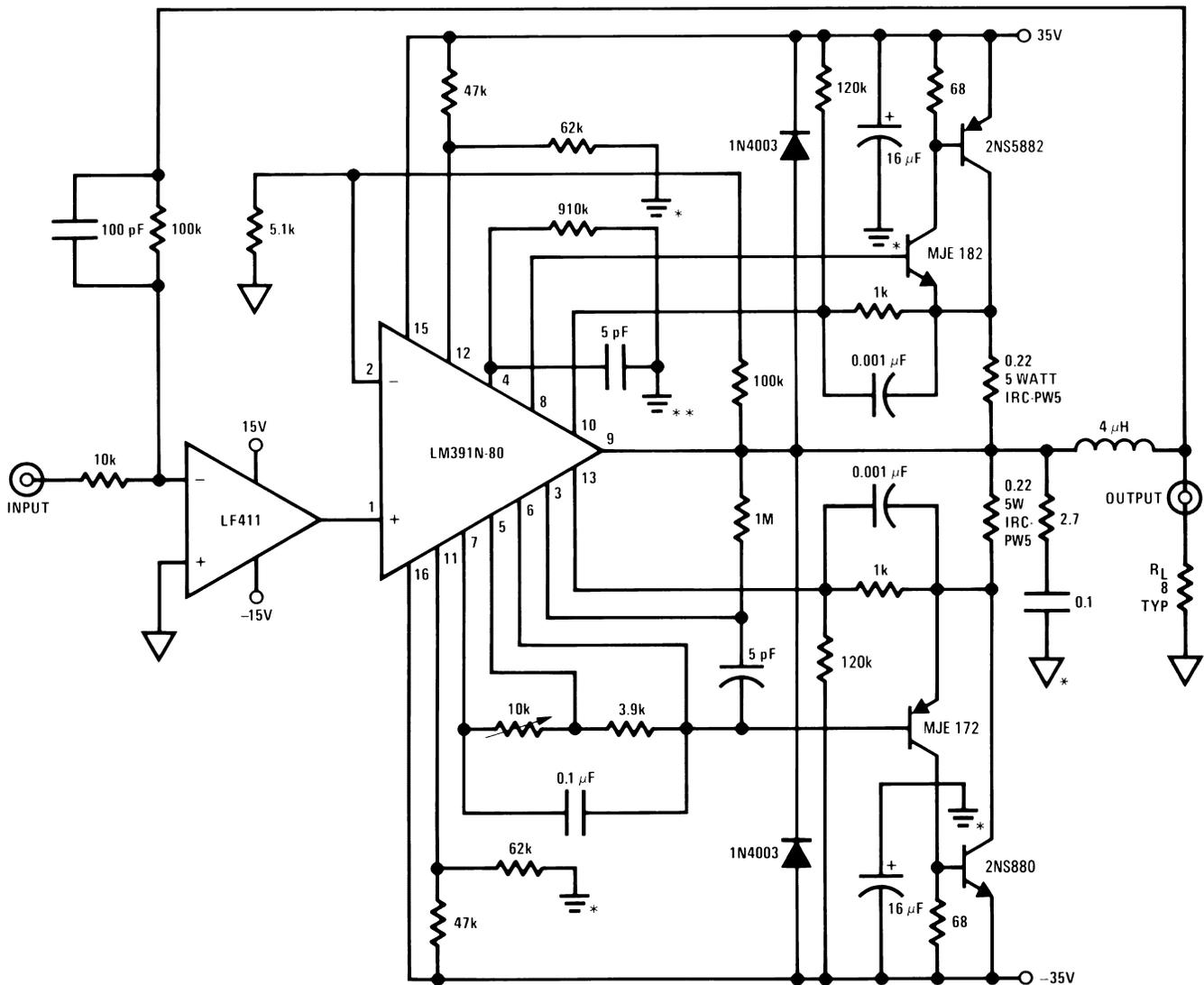
Adjust 10k pot for 25 mA zero signal current through the 0.22Ω resistors
