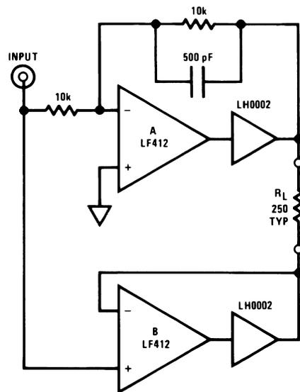
Figure 5. Double Voltage Swing Across Load Circuit
