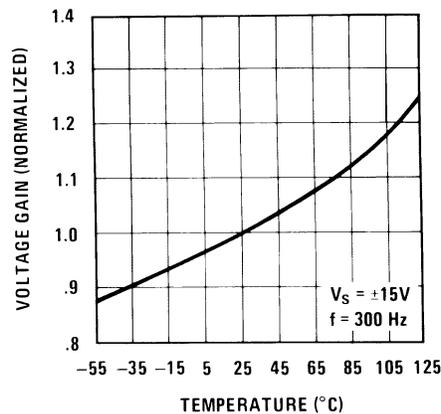
**Figure 8. Gain vs Temperature for the LM121**
