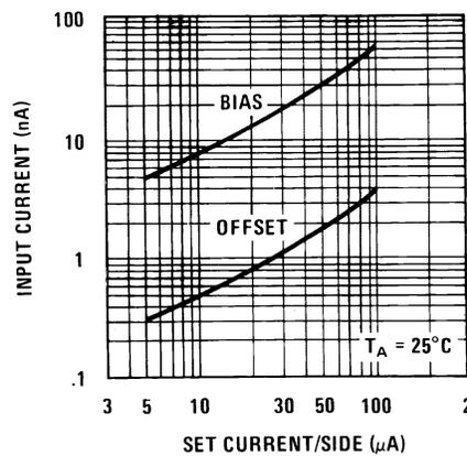
**Figure 4. Bias and Offset Current vs Set Current**
