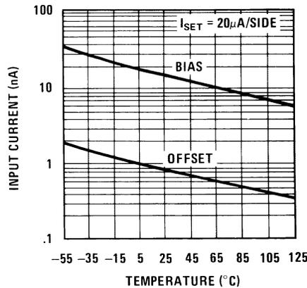
**Figure 7. Bias and Offset Current vs Temperature**
