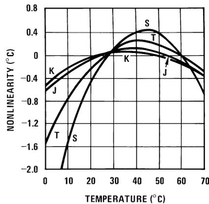
Figure 2. Thermocouple Nonlinearity
