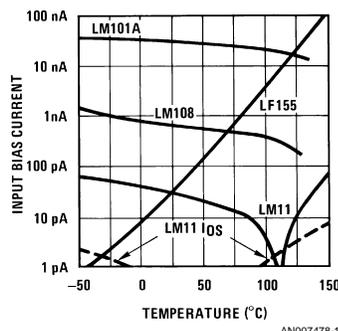
**FIGURE 1. Comparison of typical bias currents for various types of IC op amps. New bipolar device not only has lower bias current over practical temperature ranges but also lower drift. Offset current is unusually low with the new design.**
