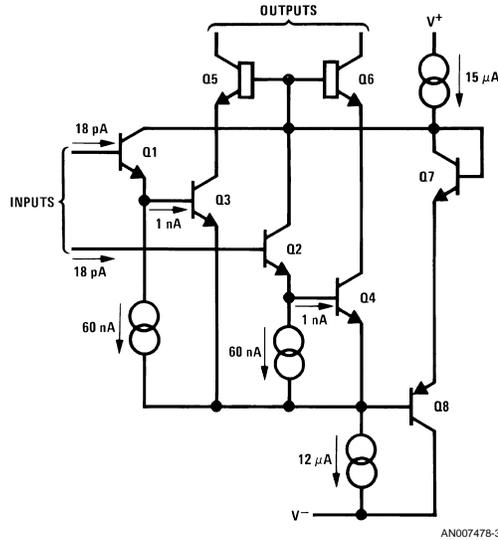
**FIGURE 3. Modifying Darlington with bleed current reduces offset voltage, drift and noise. Unique circuitry provides well-controlled current with minimal stray capacitance so that speed of the basic amplifier is unaffected.**
