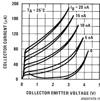
**FIGURE 13. Curve tracer display of a super-gain transistor**
