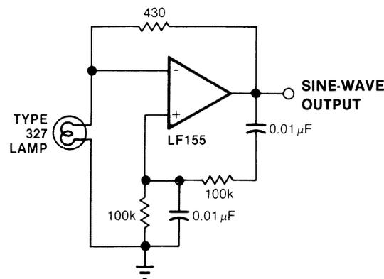
A A basic Wein bridge design employs a lamp's positive temperature coefficient to achieve amplitude stability.
