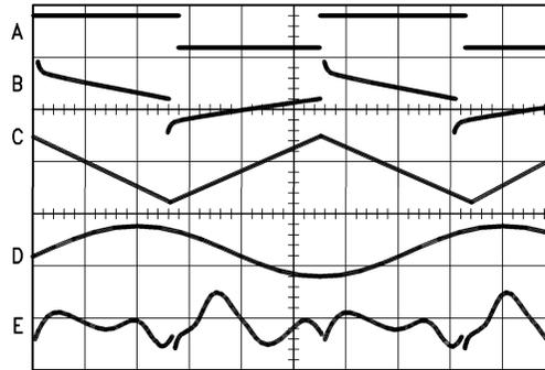
A Logarithmic shapers can utilize a variety of circuit waveforms. The input to the LF356 integrator ([Figure 14](#)) appears here as trace A. The LM311's input (trace B) is the summed result of the integrator's triangle output (C) and the LM329's clamped waveform. After passing through the 2N3810/LM394 shaper stage, the resulting sine wave is amplified by the LF351 (D). A distortion analyzer's output (E) represents a 0.35% total harmonic distortion.
