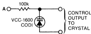
A Here, the varactor replaces the oven and retunes the crystal by changing its load capacitances.
