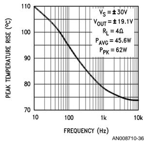
**FIGURE 29. Peak junction-temperature rise as a function of frequency with an op amp driving a resistive load under conditions of worst-case dissipation.**
