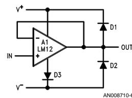
**FIGURE 2. Output clamp diodes,  $D_1$  and  $D_2$ , dump inductive-load current into the supplies when op amp goes into power limit. A third diode,  $D_3$ , may be required if the forward drop of  $D_2$  is excessive.**
