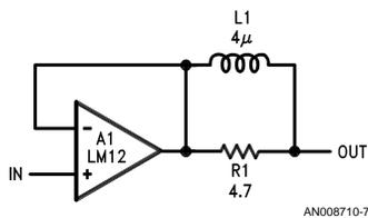
**FIGURE 3. Isolating capacitive loads with an inductor. The non-inductive resistor avoids resonance problems with load capacitance by dropping Q.**
