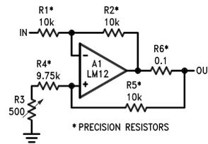
$$I_{out} = \frac{R_2 V_{in}}{R_1 R_6}$$
