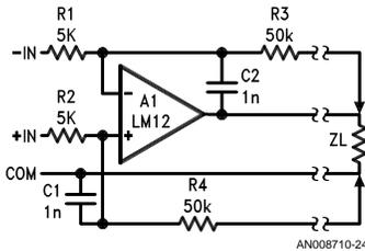
**FIGURE 22.** Remote sensing allows the op amp to correct for dc drops in cables connecting the load. Normally, common and one input are hooked together at the sending end.
