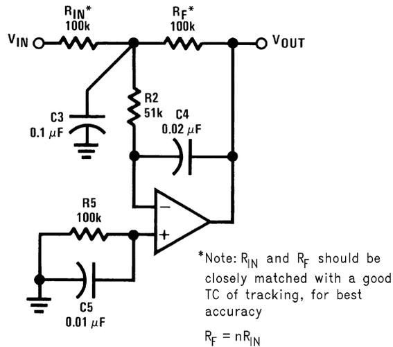
Figure 5. You Can Cascade This 2-Pole Inverting Filter Onto an F/V Converter's Output
