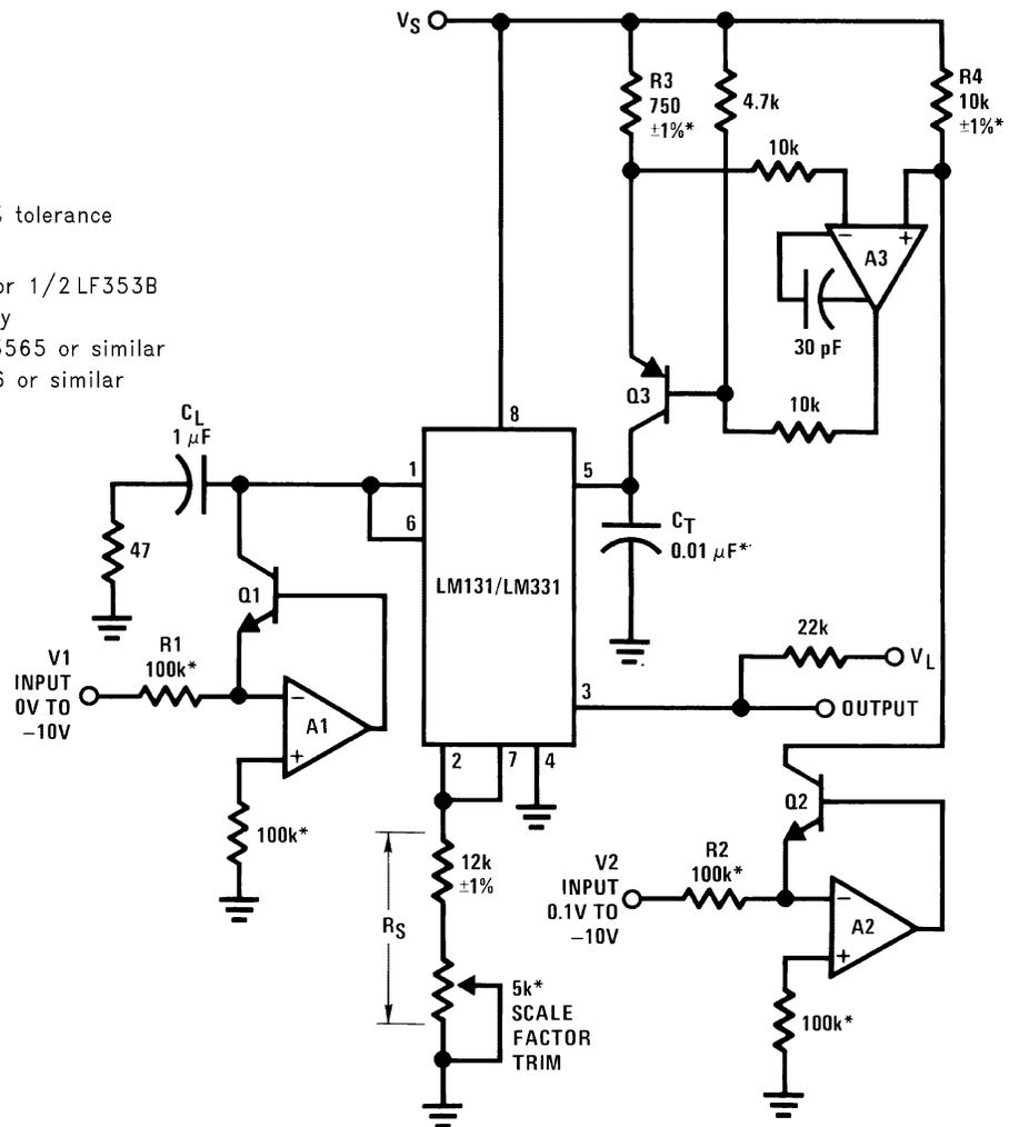
A A current pump that includes op amps A2 and A3 controls the pulse duration of the converter's internal one-shot.
