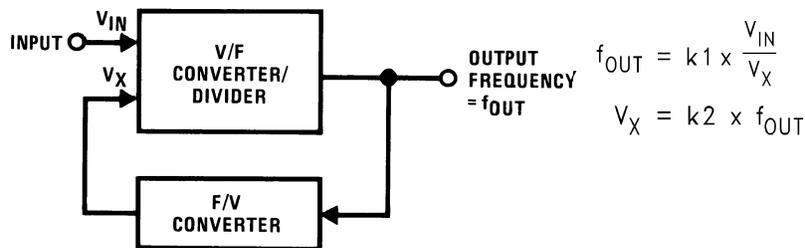
**Figure 9. Implicit Square Root Computation With V/F Converter**
