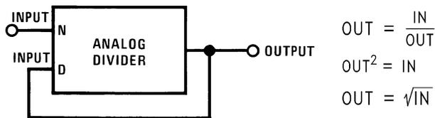
Figure 8. Implicit Square Root Computation With Analog Divider
