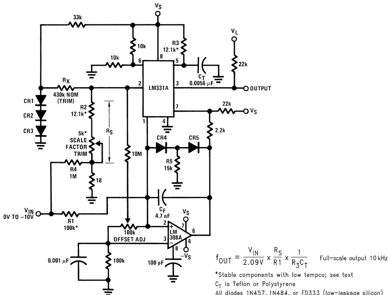
A This circuit features an ultraprecision V/F converter, capable of better than 0.02% error and 0.003% nonlinearity for a  $\pm 20^\circ\text{C}$  Range about room temperature.
