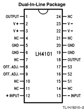
**FIGURE 1. Block Diagram and Connection Diagram of LH4101**
