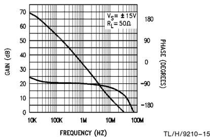
FIGURE 10. Bode Plot of LH4101,  $V_S = \pm 15V$
