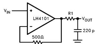
FIGURE 12. Compensation for Capacitive Load
