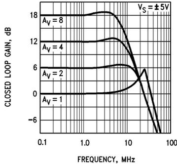
FIGURE 13. Closed Loop Frequency Response,  $V_S = \pm 5V$
