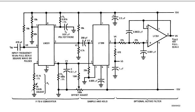
FIGURE 2. Improved F-to-V Converter Using Sample-and-Hold
